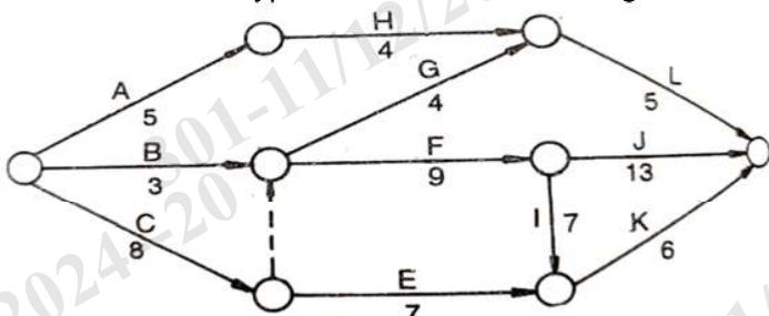
l) Determine the aggregate resources requirement, period by period for the network given below. The figures over the arrow indicate the duration of the activities and figures below the arrow indicate requirement of mason for the project. Use resource smoothing technique to maintain the mason requirement of 2.
