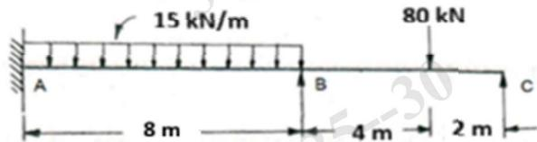
f) Determine the collapse load for the fixed beam shown below having plastic moment capacity 150 kNm.
