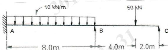
f) Determine the collapse load for the fixed beam shown below having plastic moment capacity  $M_p$ .
